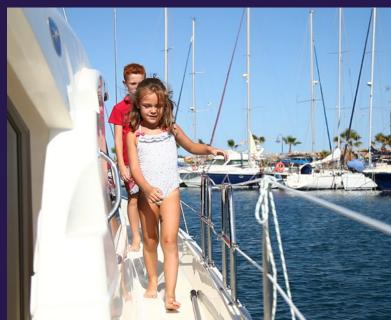
The Alabtross 42 has wide side-decks which can be accessed from the helm position without having to climb over the cockpit combing.
